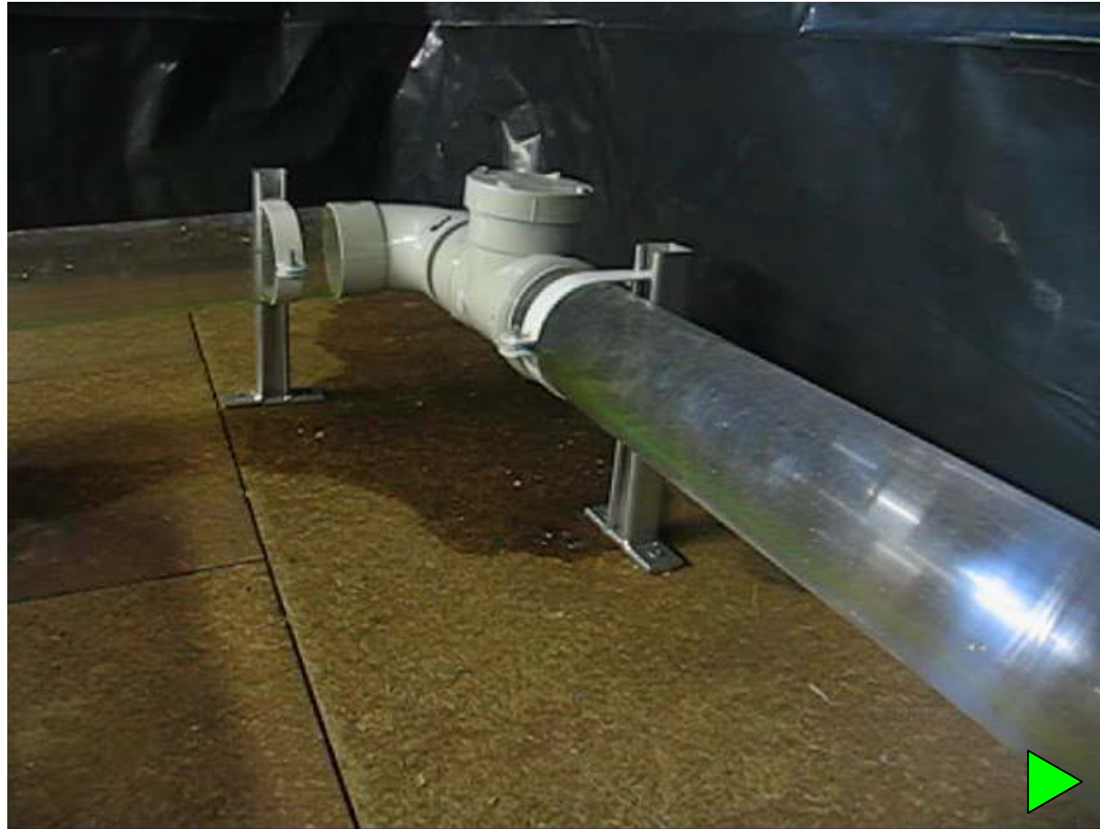
The affects of 90 degree bends (short radius)
