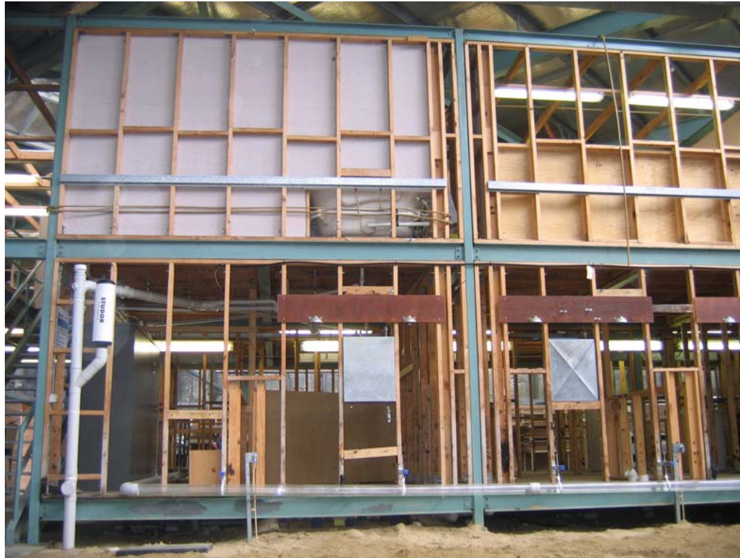
Canberra Institute of Technology (CIT) drainline simulation test rig
