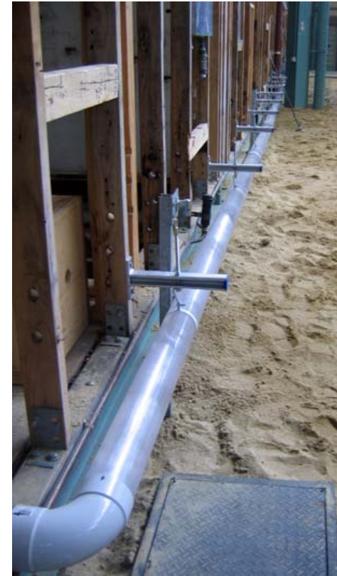
Canberra Institute of Technology (CIT) drainline simulation test rig
