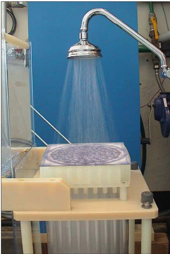
New Low-flow shower performance testing – Spray Coverage
